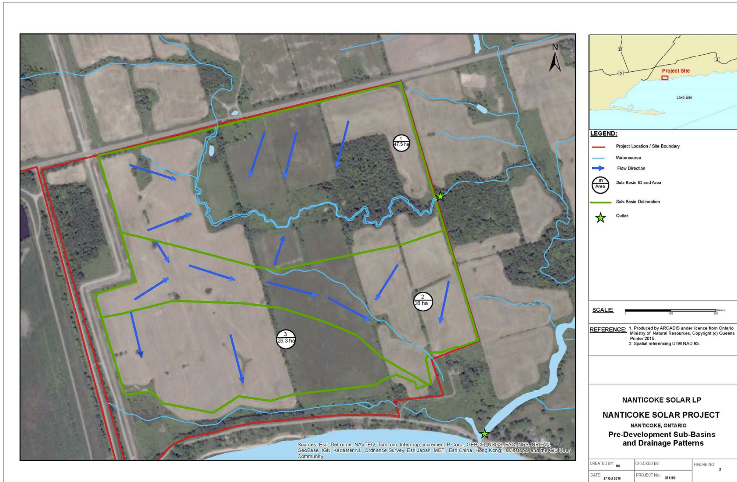
Figure 5 – Pre-Development Surface Water Drainage
