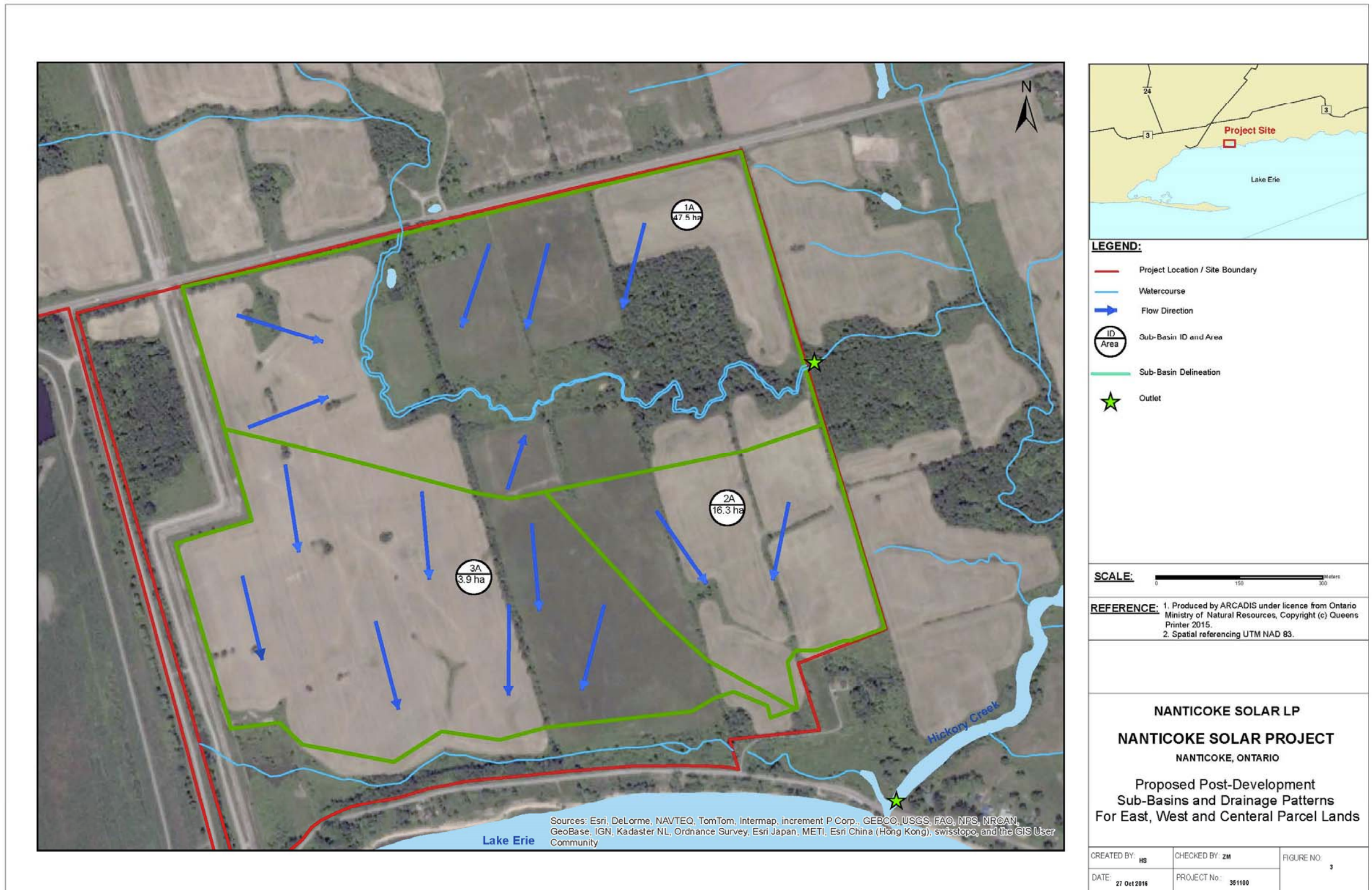
Figure 6 – Post-Development Surface Water Drainage
