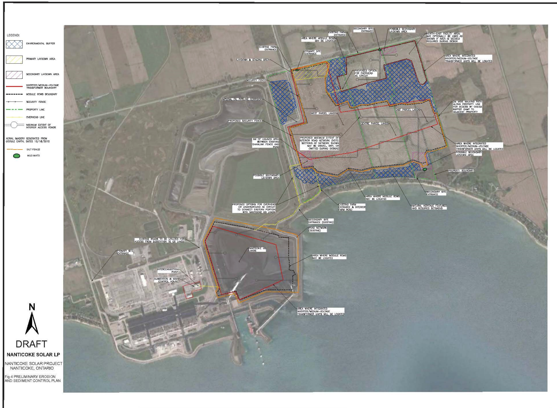
Figure 4 – Preliminary Erosion and Sediment Control Plan
