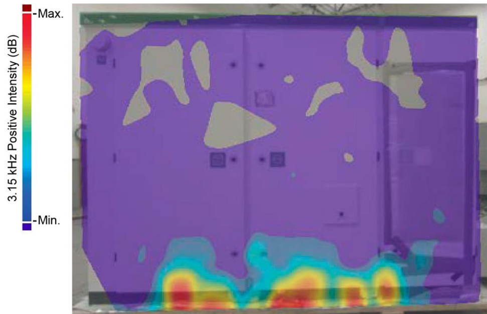
Figure 4 LV and Communications end (3.15 kHz, switching frequency)
