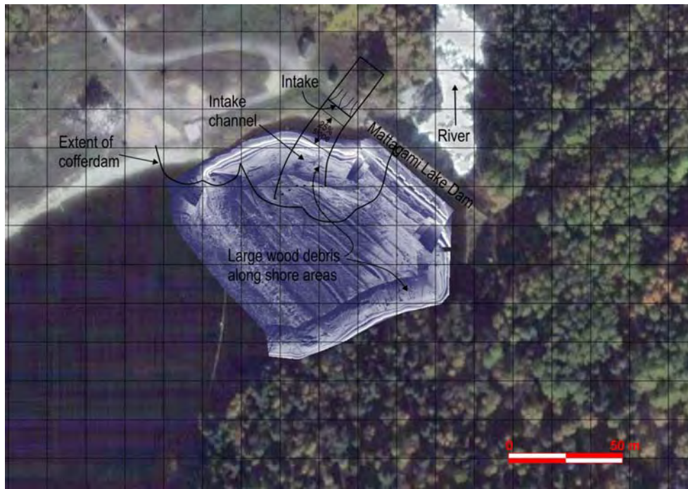
Figure 3.2 Side-scan Sonar Image of Mattagami Lake Adjacent to the Mattagami Lake Dam
