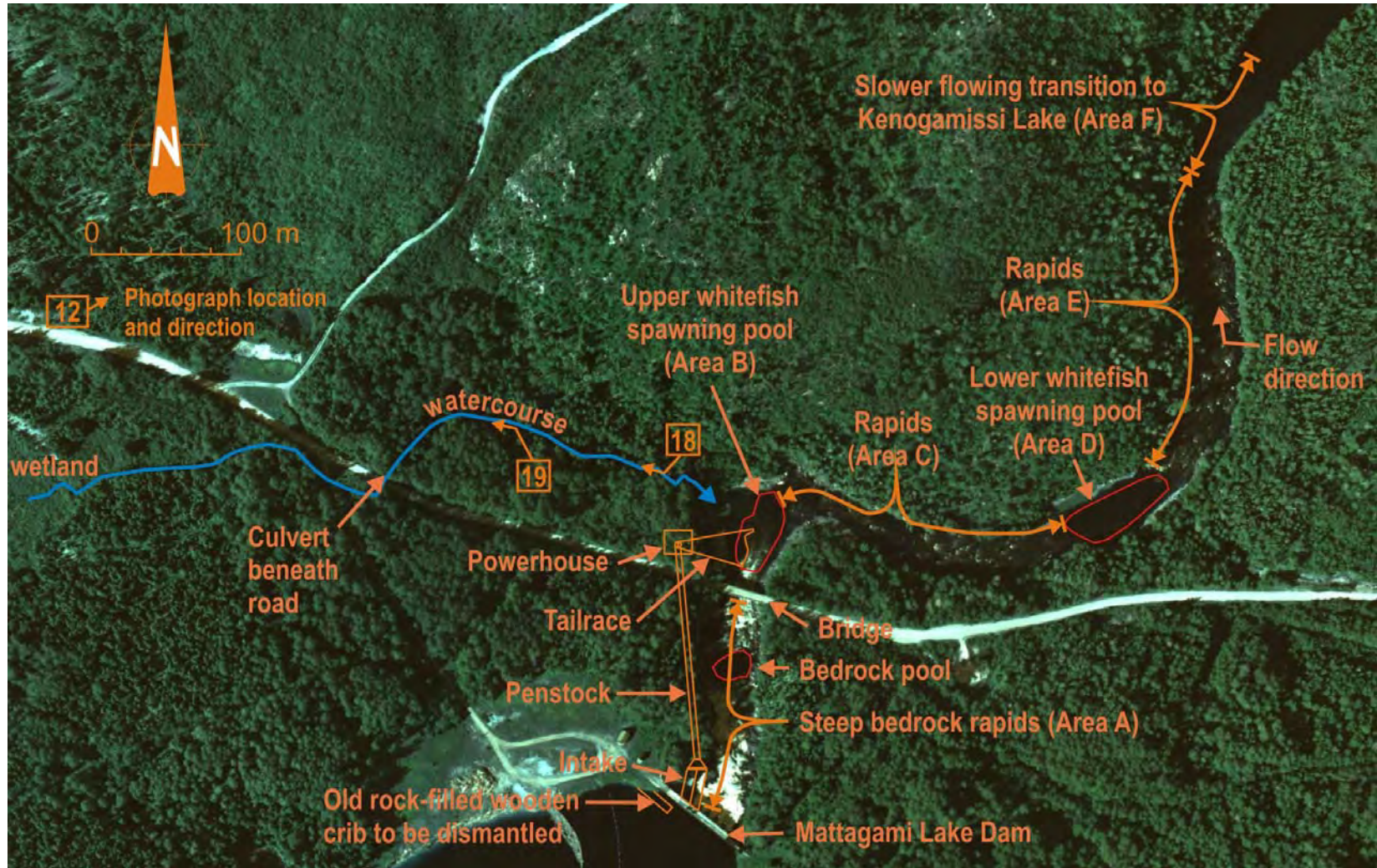
Figure 3.9 Project Study Area from Mattagami Lake to Kenogamissi Lake, Showing the Main Site Features, the Location and Basic Layout of the Proposed Undertaking, Watercourse Sections Referenced in this Report, and the Location of Photographs of the Small Watercourse Flowing from the West
